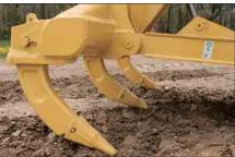
**Multi-Shank Ripper.** The multi-shank parallelogram ripper offers the choice of one, two or three shanks depending on job conditions. Curved or straight ripper shanks are available.
