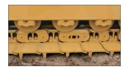
Roller Design. The SystemOne<sup>™</sup> roller has a taller flange to improve track guiding, especially in sidesloping applications. Advanced features and reduced piece parts enhance the rollers which help eliminate any flexing in the collars and avoid oil loss. The roller is maintenance-free and serviced as a group only. To achieve total balanced wear, carrier rollers with increased wear life are also used.
