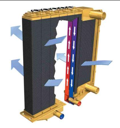
**Serviceability.** This modular core design permits removal of a single core without removing the entire radiator so repair costs and downtime are reduced. The top tank, side channels and one sealing surface makes AMOCS more reliable and easier to service. A site gauge allows for quick service checks.
