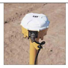
**AccuGrade GPS.** AccuGrade GPS computes the positioning information on the machine, compares the position of the blade relative to the design plan and delivers that information to the operator via an in-cab display.
