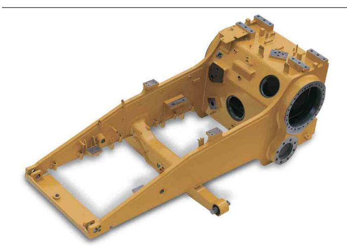
**Frame and Castings.** The D6T III frame is built to absorb high impact shock loads and twisting forces. The frame has a reinforced saddle and a welded front cross-member that add strength to the frame to better handle lateral and twisting forces. Steel castings augment the strength of the main case.
