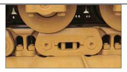
**Master Link.** A unique feature of the SystemOne Undercarriage is that, unlike traditional undercarriage, a master style link is not required. This improves track reliability and durability. The unique straight link design allows the track to be taken apart at any joint by using the proper Caterpillar tooling to press the link on or off.
