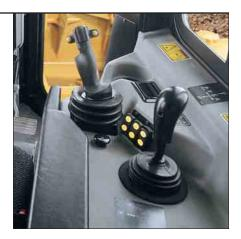
**Dozer Control Lever.** The D6T features ergonomically designed dozer controls with low-effort, pilot-operated hydraulics for added operator comfort, easy operation and precise work tool control. When equipped with a VPAT blade, the blade control allows simultaneous six-way control of the blade with a thumb rocker control to adjust blade angle. The dozer control is changed to an electro-hydraulic control when the AccuGrade<sup>®</sup> Ready Option is installed.
