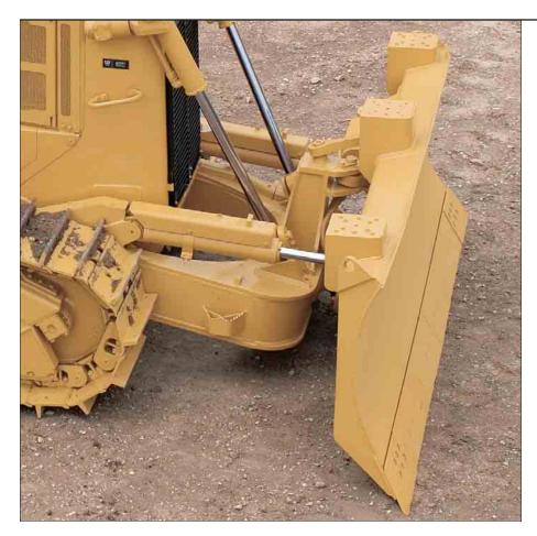
**Cat Blades.** All blades feature a strong box-section design that resists twisting and cracking. Blades are made of Cat DH-2<sup>™</sup> steel that has high tensile strength and stands up to the most severe applications. Heavy moldboard construction and hardened bolt-on cutting edges and end bits add strength and durability.
