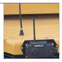
**Cat® Product Link.** When machines are operating at several different job sites, it becomes more difficult to keep current and accurate records. That can lead to missed maintenance, poor use of assets and wasted time. Product Link provides two-way information flow between machine on-board systems and your desktop computer through Dealer Store Front and Equipment Manager. Cat Product Link enables the use of Equipment Manager to keep you in touch with your machines.
