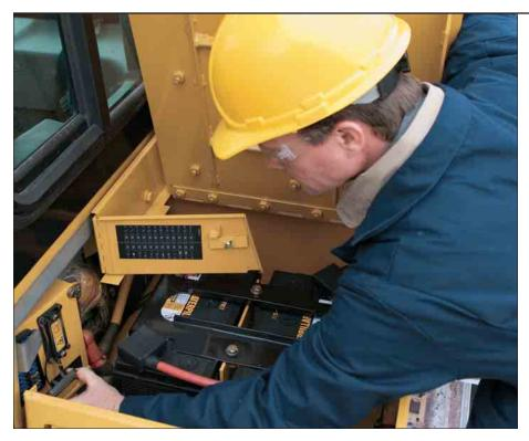
**Built-in Serviceability.** Major D6T components are made as modules and most can be removed without disturbing or removing others. This means less service time and more productivity.
