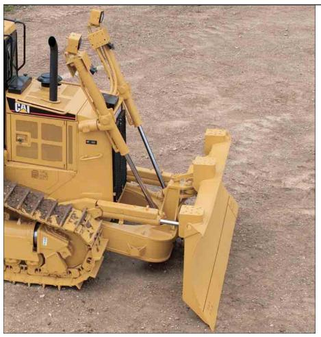
**Cat Blades.** All blades feature a strong box-section design that resists twisting and cracking. Blades are made of Cat DH-2<sup>™</sup> steel that has high tensile strength and stands up to the most severe applications. Heavy moldboard construction and hardened bolt-on cutting edges and end bits add strength and durability.
