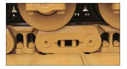
Master Link. A unique feature of the SystemOne Undercarriage is that, unlike traditional undercarriage, a master style link is not required. This improves track reliability and durability. The unique straight link design allows the track to be taken apart at any joint by using the proper Caterpillar tooling to press the link on or off.
