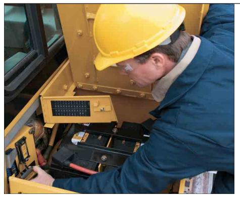
**Built-in Serviceability.** Major D6R Series III components are made as modules and most can be removed without disturbing or removing others. This means less service time and more productivity.
