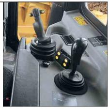
Dozer Control Lever. The D6R Series III features ergonomically designed dozer controls with low-effort, pilot-operated hydraulics for added operator comfort, easy operation and precise work tool control. When equipped with a VPAT blade, the blade control allows simultaneous six-way control of the blade with a thumb rocker control to adjust blade angle. The dozer control is changed to an electro-hydraulic control when the AccuGrade® Ready Option is installed.
