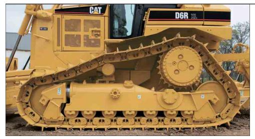
**SystemOne Undercarriage.** The exclusive SystemOne Undercarriage is designed for reliability and durability by greatly increasing undercarriage life and reducing owning and operating costs.
